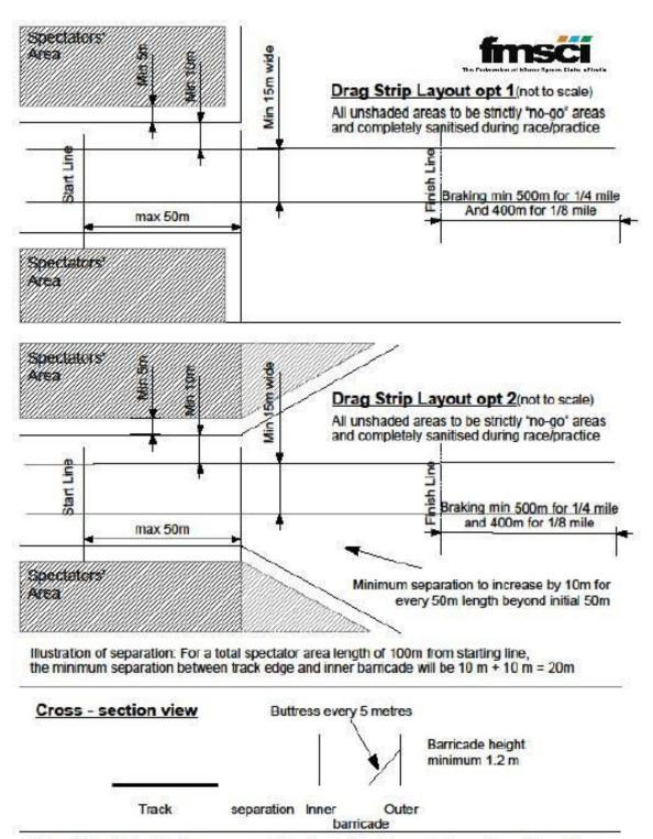
Notes: (i) Double barricading recommended, not mandatory for spectator area beyond run off area; (ii) barricades not required in case of masonry wall.
